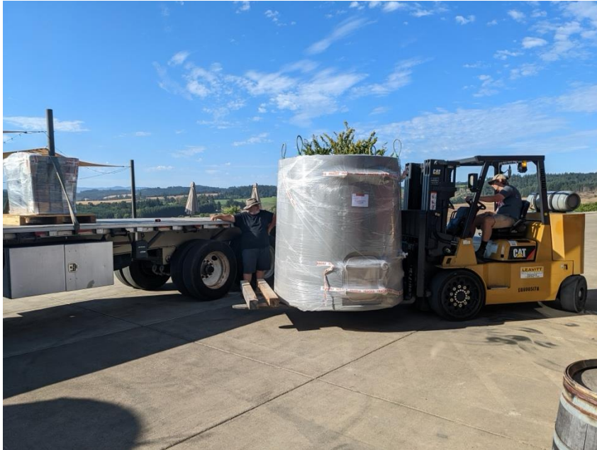
Lifting ACL32 with 12k Vertical Mast (warehouse) Forklift – Preferred Equipment
