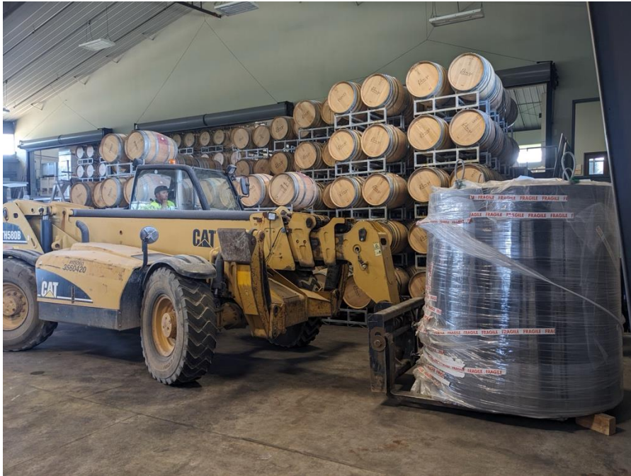
Lifting ACL32 with 12k Telehandler Forklift (less ideal equipment)
